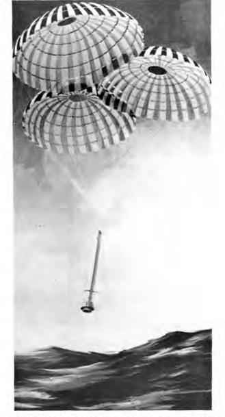
DRAWING shows one of the booster rockets of the space shuttle with full deployment of the main parachute array. Sandia is aiding NASA with the design and development of the recovery system for space shuttle booster rocket.
